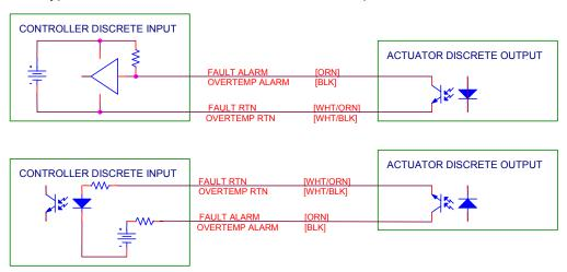
Figure 2-6: Typical Fault Alarm Connection
